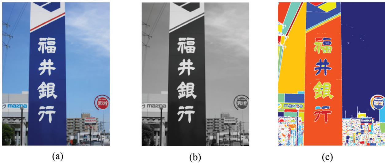
Figure 2. An example for natural scene image segmentation (a) Original Image, (b) Grayscale Image, (c) Labeling Image for Homogeneous Regions.
