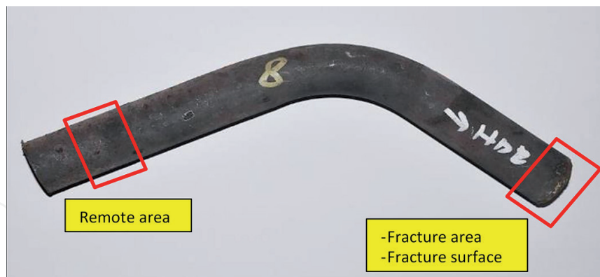
Figure 9. Dimensional reference of oxide thickness measurement.
