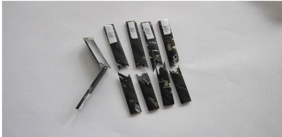
Figure 1. Example: Low strength of the fiber composite structure due to the poor joint of the fiber with matrix.
