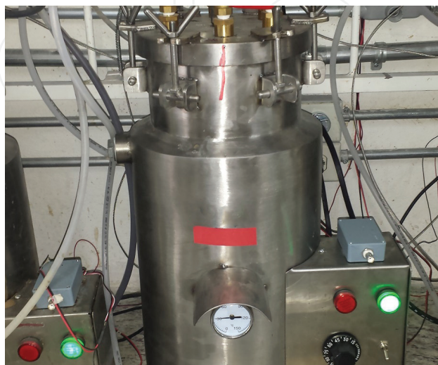
Figure 1. Laboratory-scale anaerobic reactor with pumped circulation.
