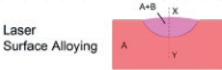
Figure 3. Schematic diagram displaying laser surface alloying [15].
