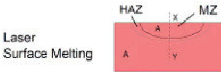
Figure 2. Schematic diagram illustrating the heat-affected zone and melt zone created by laser surface melting [15].
