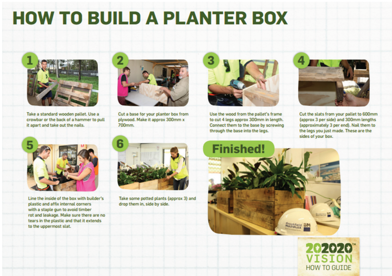
Figure 4. Steps involved in constructing a planter box from recycled materials.
