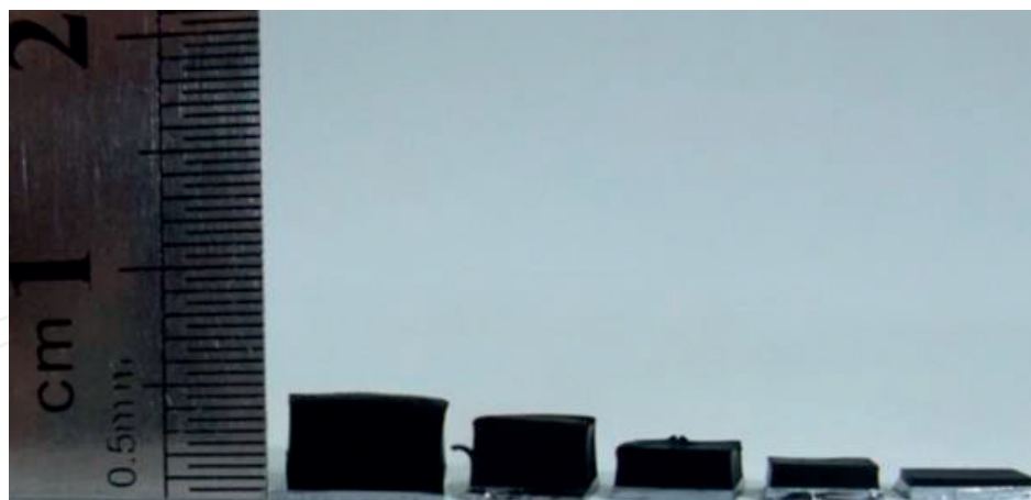
Figure 3. Depicting the lengths of VACNTs grown with growth time of 3 h, 2 h, 1 h 30 min 10 min (reprint from Ref. [22] with permission).
