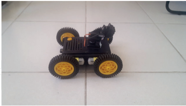
Figure 7. Robot based on Raspberry pi used for experiments.
