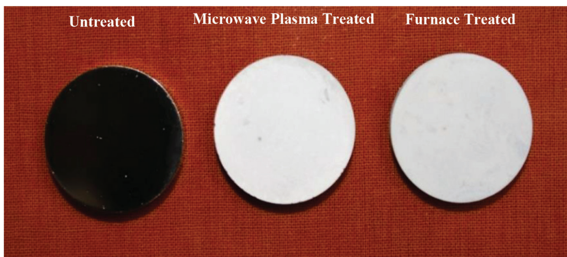
Figure 9. Photograph of oxide-layer formed on the 25-mm diameter titanium disc using microwave plasma and air furnace. Reprinted from [64] with permission from Elsevier.
