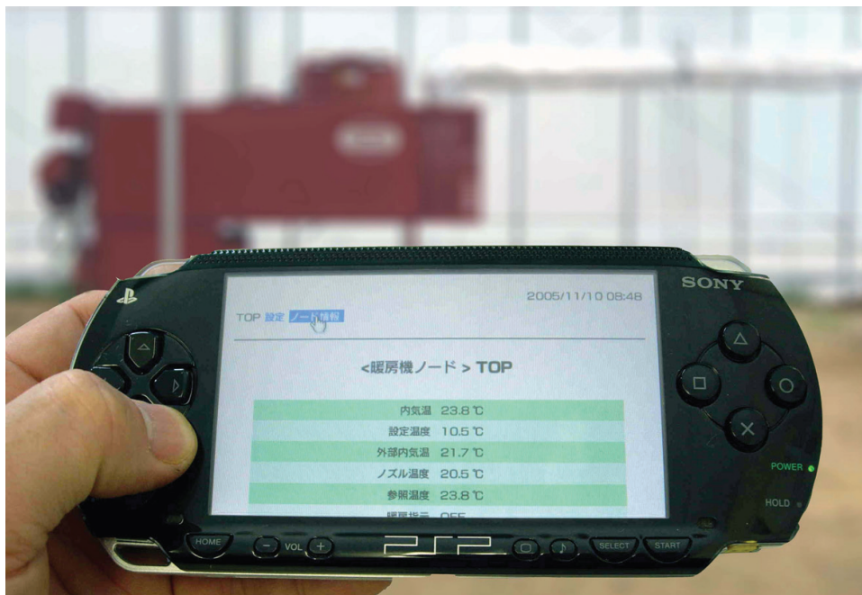
Figure 4. Managing the node for an oil air heater using a portable game console in a greenhouse using an UECS.
