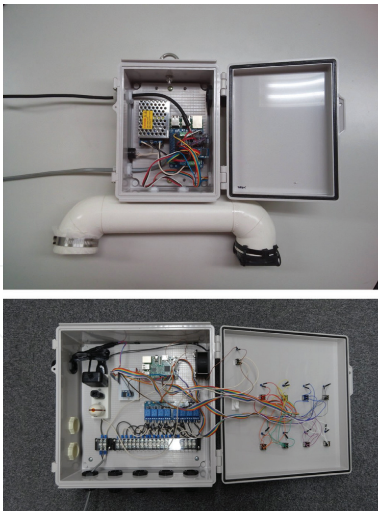
Figure 9. The UECS DIY node completed by the workshop. Upper: sensor node for measuring greenhouse climate, lower: relay node for controlling actuators such as open-close motor of roof ventilators.
