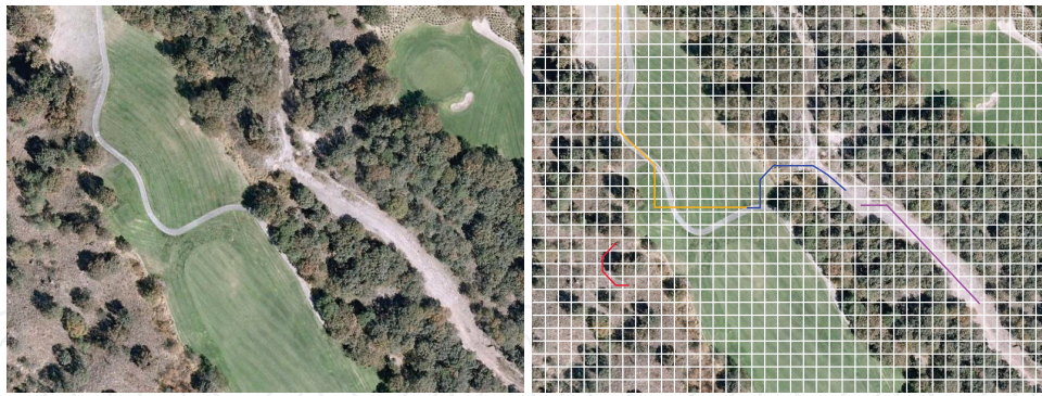
Figure 1. Left: Satellite like image. Right: Grid cells and lines with different colours representing sample paths.
