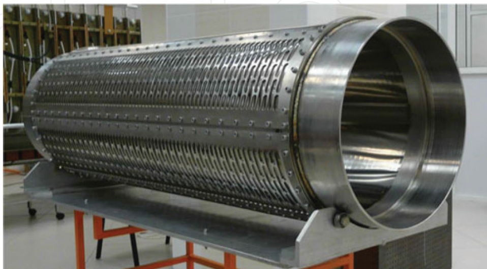
Figure 14. Gas chamber of the XeF(C-A) amplifier with windows for electron beam injection.
