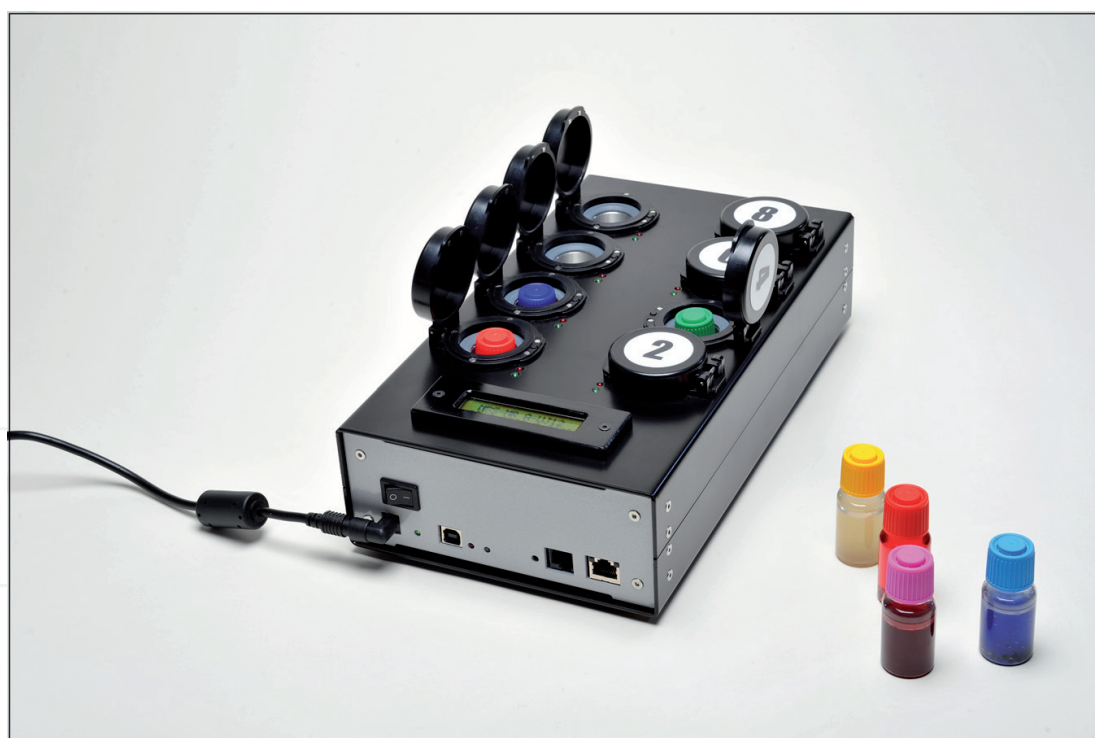
Figure 1. MBS “UTI CHECK.” MBS “UTI CHECK” is an automated colorimetric culture-based test. It is composed by mono-use, disposable and ready-to-use reaction vials (right) in which 1 ml of urine can be inoculated without any preliminary treatment. Up to eight urine-inoculated reaction vials can be independently allocated in an automatic thermostated optical reader (left) that it is able to detect color change induced by the growth of bacteria and automatically correlates the time required for color change with the number of bacteria present in the urine samples. Different vials contain selected antibiotics and the occurrence of the color change in the presence of antibiotics indicates antibiotic resistance of bacteria present into the urine sample.
