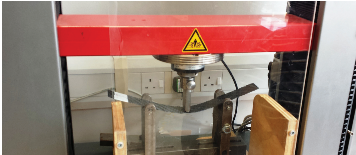
Figure 1. Flexural test equipment: universal testing machine.
