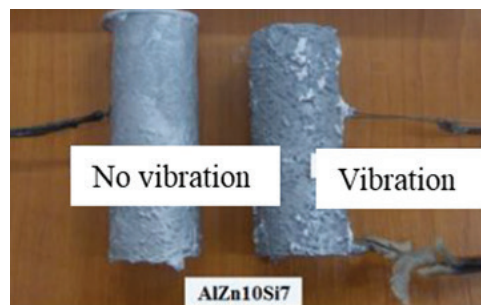
Figure 16. Photographs showing the roughness of the samples in AlZn10Si7 alloy with and with no vibration [10].
