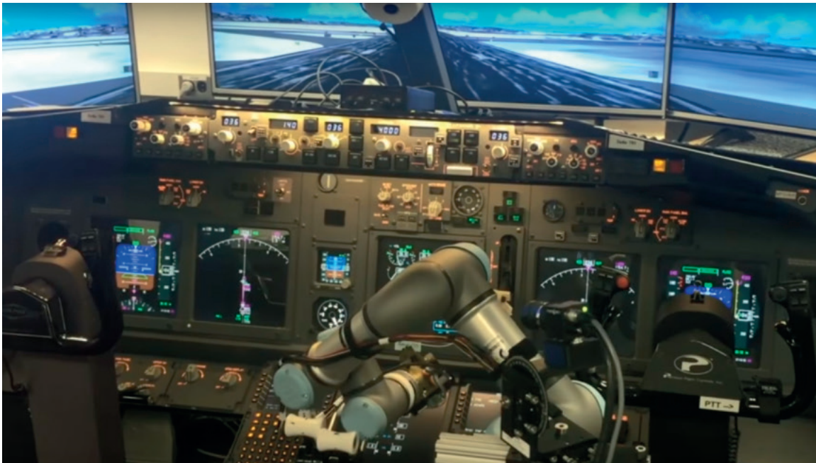
Figure 1. Robotic co-pilot ALIAS landing a Boeing 737.
