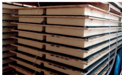
Well-insulated airtight wall panels backed with boards of rigid polyurethane foam
