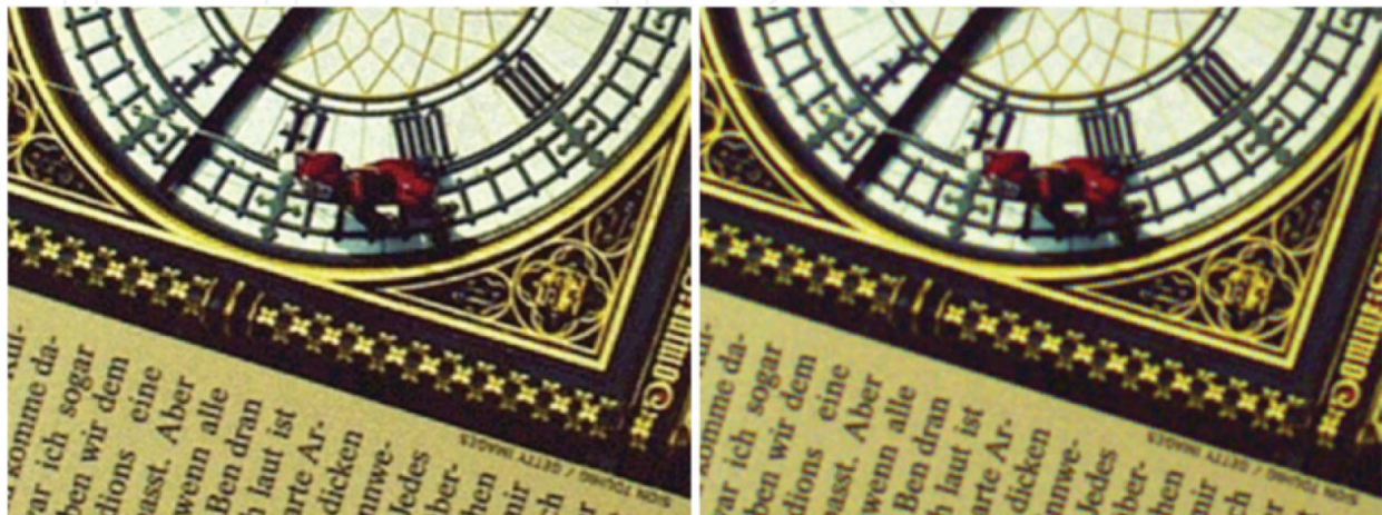
Figure 18. SmartGreen3 color reconstruction followed by false color detection, edge enhancement, and bilinear interpolation (left). Standard color reconstruction followed by edge enhancement and bilinear interpolation (right).
