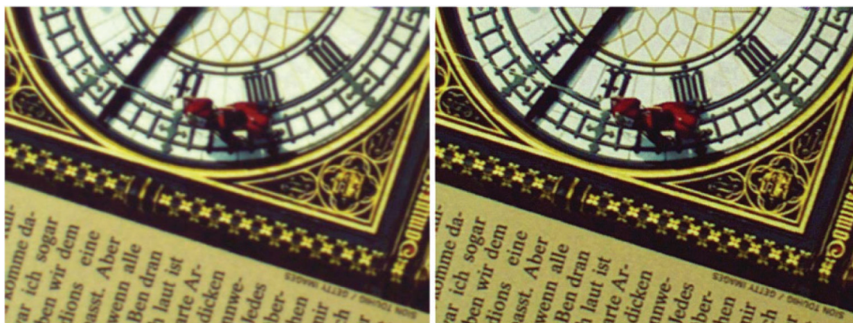
Figure 19. Super-resolution reconstruction and zoom (left). Super-resolution reconstruction, zoom, and edge enhancement (right).
