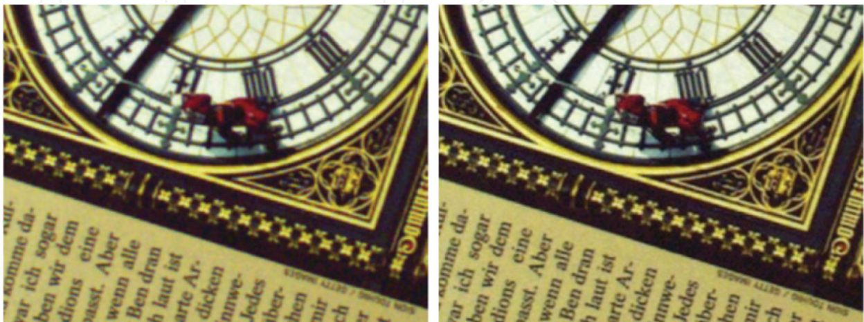
Figure 17. Standard color reconstruction and bilinear interpolation (left). SmartGreen3 color reconstruction followed by false color detection and bilinear interpolation (right).
