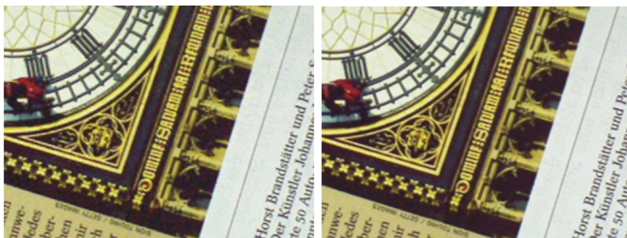
Figure 8. SmartGreen1 reconstruction with SR of “paper,” frame 1 (left) and frame 20 (right). For the first frame, no SR is possible, and so it is equal to bilinear interpolation.
