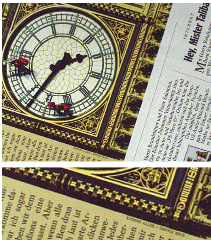
Figure 14. SmartGreen3 color reconstruction with false color detection and edge enhancement.
