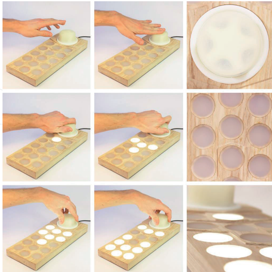
Figure 6. Design four: rotary relays. PPP 3D print, wood, Arduino microcontroller, potentiometer, and LED lights.
