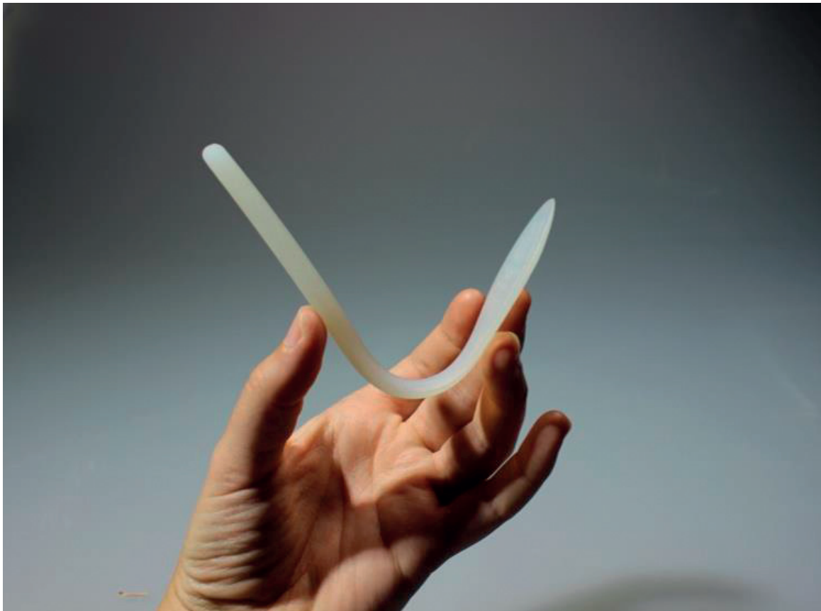
Figure 9. 3D printed prototype to test bending.
