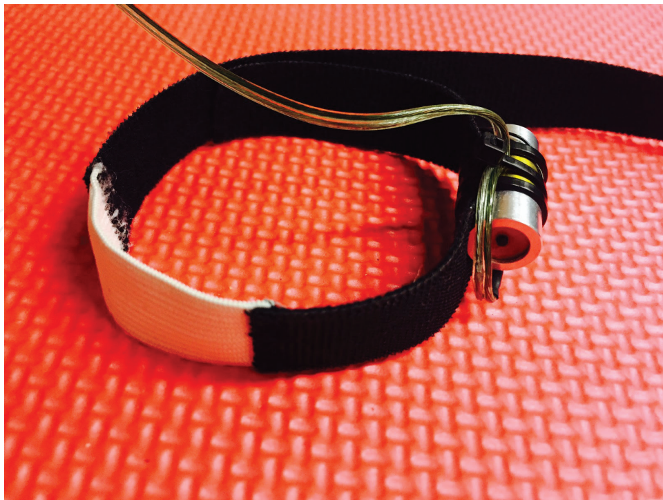
Figure 1. The vibrating band used in the study consists of a Haptuator attached to a Velcro strap.
