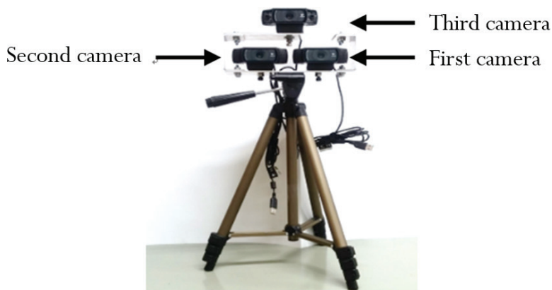
Figure 6. Image input device using three web cameras.
