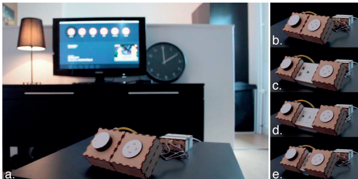
Figure 6. Adaptive remote control by Paul van Beek, 2014 (Photos courtesy of Paul van Beek). (a) The adaptive remote control in context (closed state); (b–e) Depending on the requirements of the task the remote control opens and gives context dependent controls on the slider in the middle.
