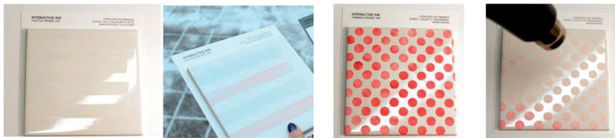
Figure 8. Thermochromic pigments were painted on ceramic surfaces: these patterns are responsive to differences in temperature, such as cold or heat.
