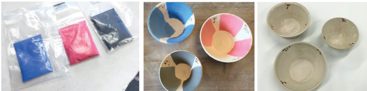
Figure 7. Thermochromic pigment powder was added to the glazing base at different concentration for glazing ceramics. However, the thermochromic glaze lost its properties under high heat during the baking process in the kiln.
