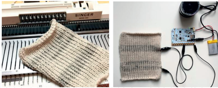
Figure 12. Conductive fibers were knitted together with regular yarn to create conductive areas for touch interactivity to generate output, such as sound in this example.
