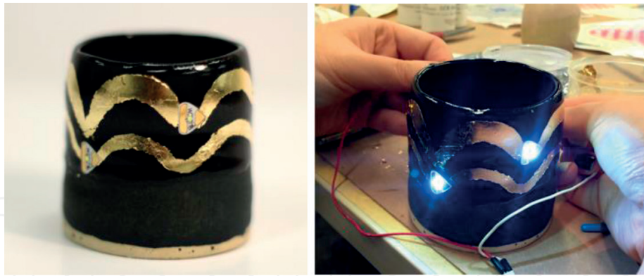
Figure 10. Testing of adding simple LED light interactivity using gilded metallic circuits.
