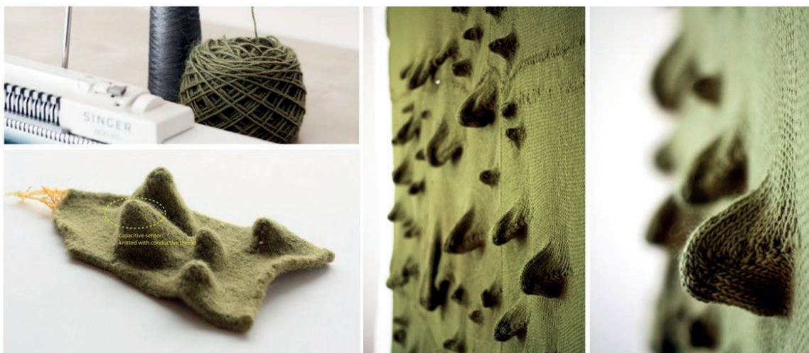
Figure 4. Knitting with two different types of yarn to create a conductive 3D structure knit. Conductive fibers are embedded in each tip of the three-dimensional forms.
