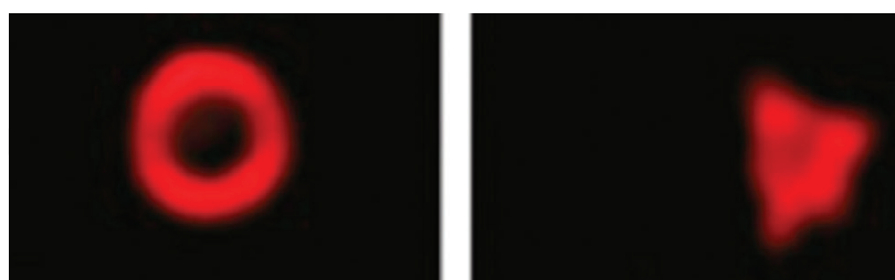
Figure 10. Fluorescence images of a giant anchored PNIPA lipobead below (left) and above (right) T_v . Red images originated from 0.05 mol% RhodB-PE component within the lipid bilayer. The images were adopted from [25, 28].
