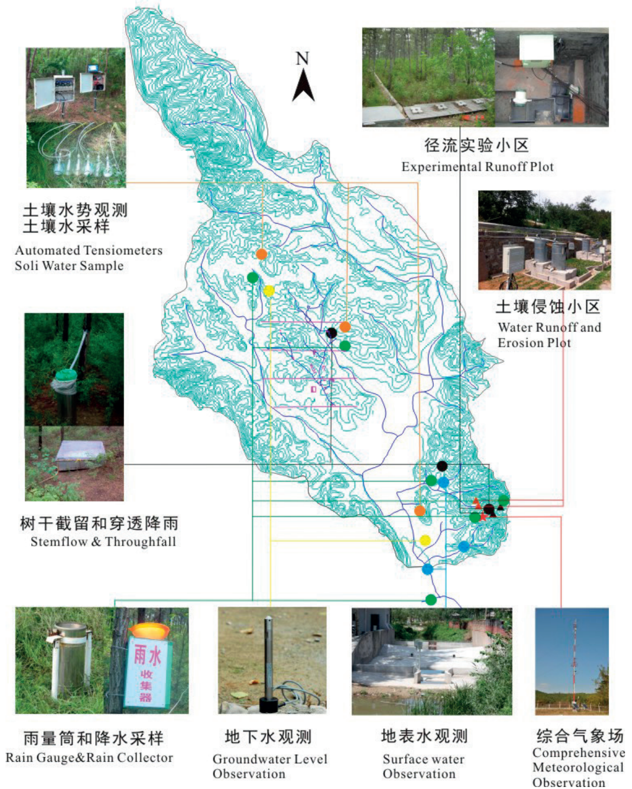
Figure 3. Layout of Chongling catchment showing the location of instruments.
