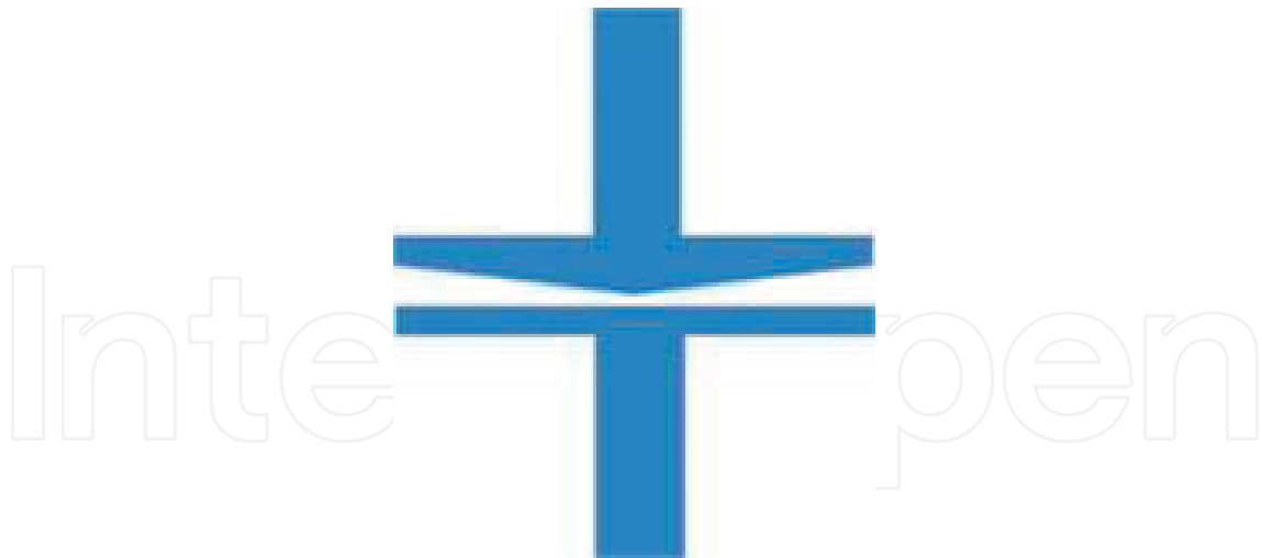
Figure 27. Cone plate of rheometer.
