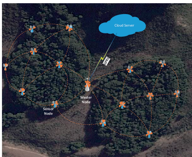
Figure 8. WSN mesh network architecture.
