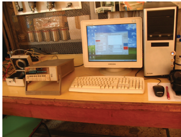
Figure 10. Stand for surface and volume resistivity measurements.
