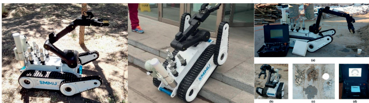
Figure 6. The biochemical sampling robot and tests.
