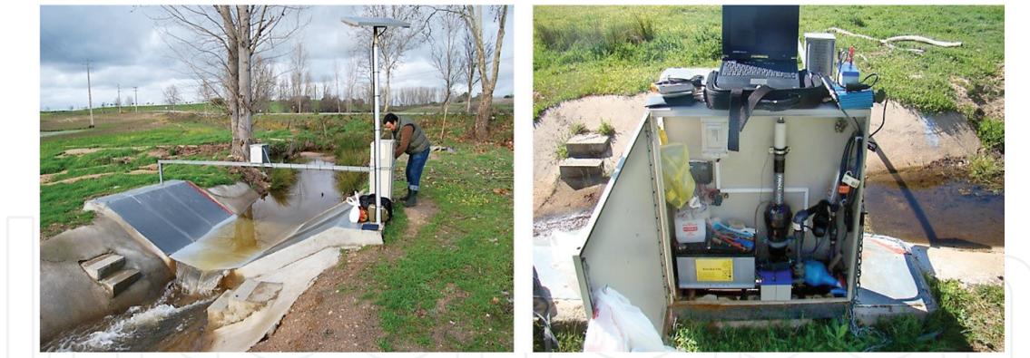
Figure 8. Hydrometric and water quality station located at the outlet of the study catchment.
