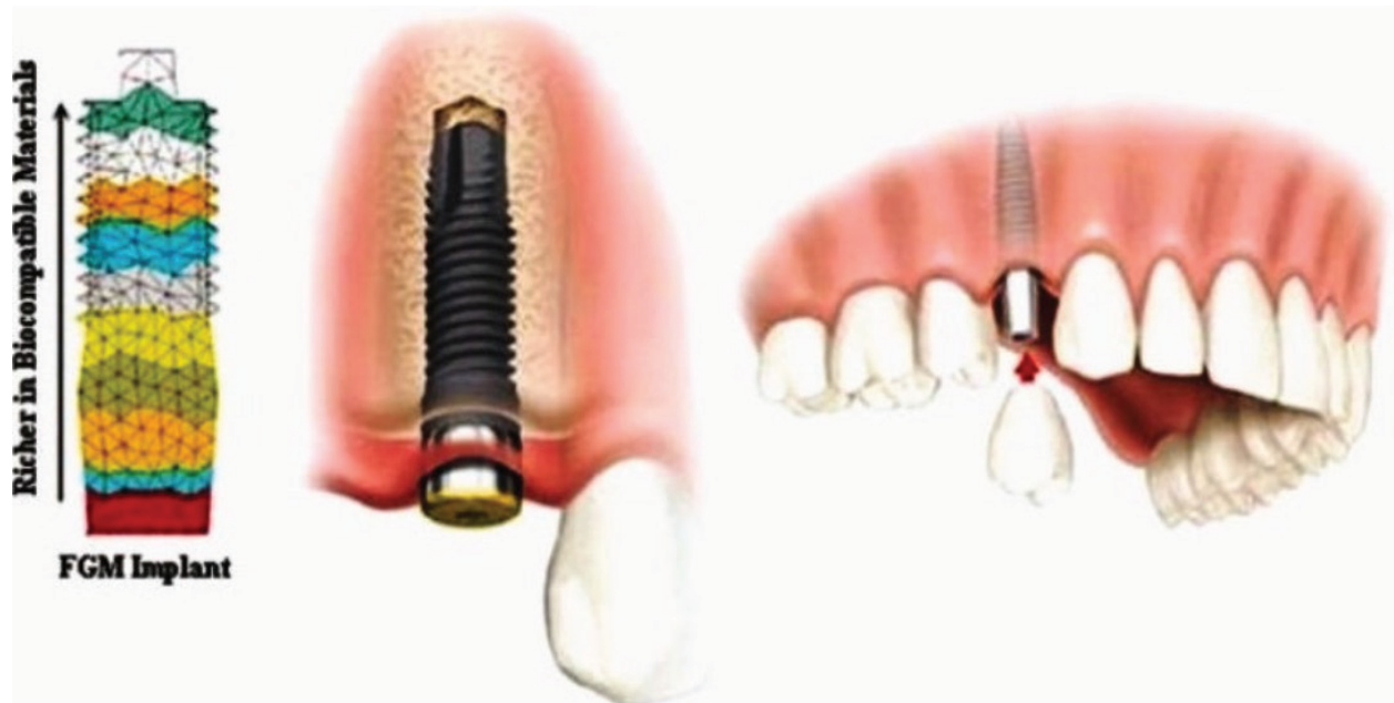
Figure 1. FGM dental implant with graded material composition.
