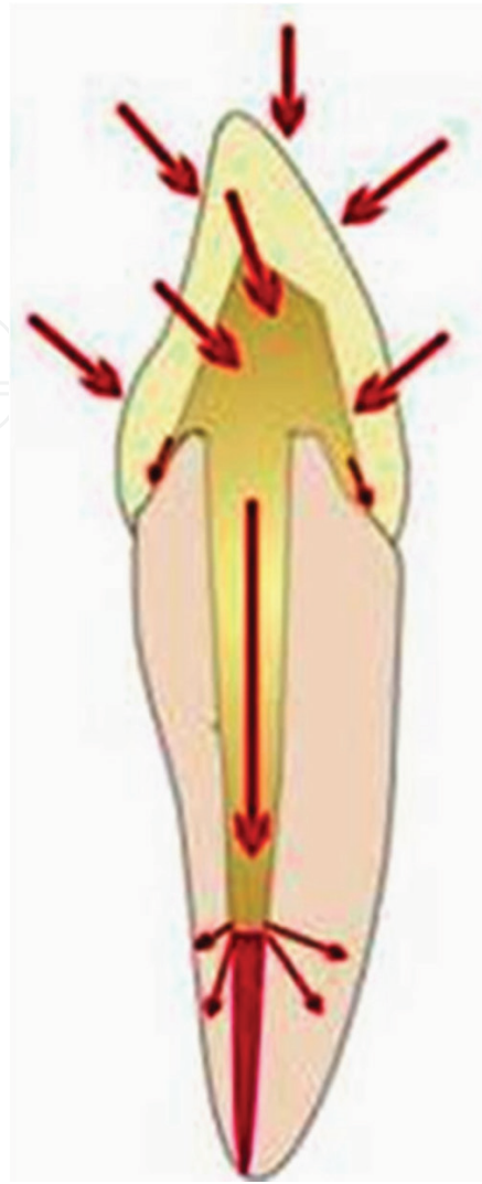
Figure 4. Stress concentration due to commercial dental post.
