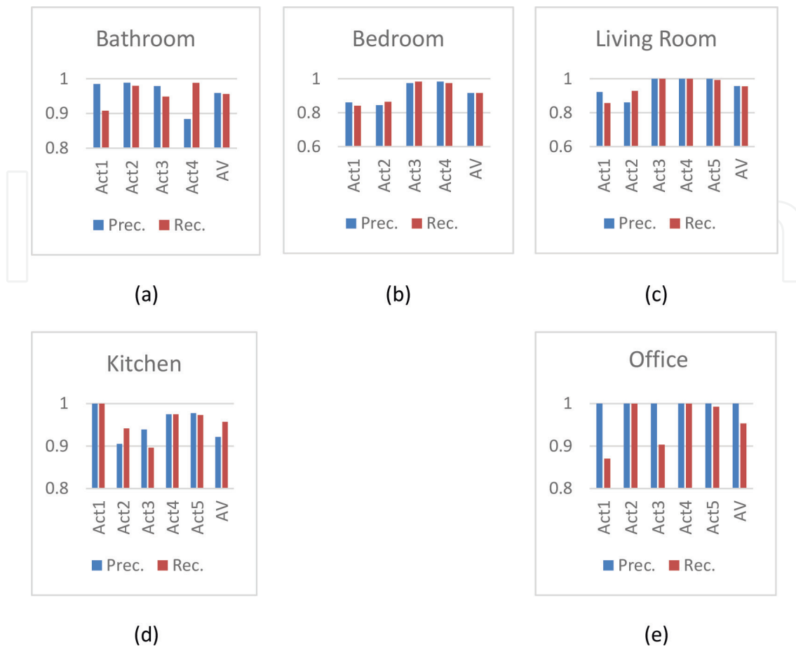
Figure 8. Performance on the CAD-60 ('new person'). Results are reported in terms of precision (Prec) and recall (Rec) and an average (AV) per scenario. Overall AV: precision 94.83%; recall: 94.74%. Activities in (a): Act1—rinsing water; Act2—brushing teeth; Act3—wearing lens; Act4—random + still; activities in (b): Act1—talking on phone; Act2—drinking water; Act3—opening container; Act4—random + still; activities in (c): Act1—talking on phone; Act2—drinking water; Act3—talking on coach; Act4—relaxing on coach; Act5—random + still; activities in (d) Act1—drinking water; Act2—cooking chopping; Act3—cooking stirring; Act4—opening container; Act5—random + still; activities in (e): Act1—talking on phone; Act2—writing on whiteboard; Act3—drinking water; Act4—working on computer; Act5—random + still.
