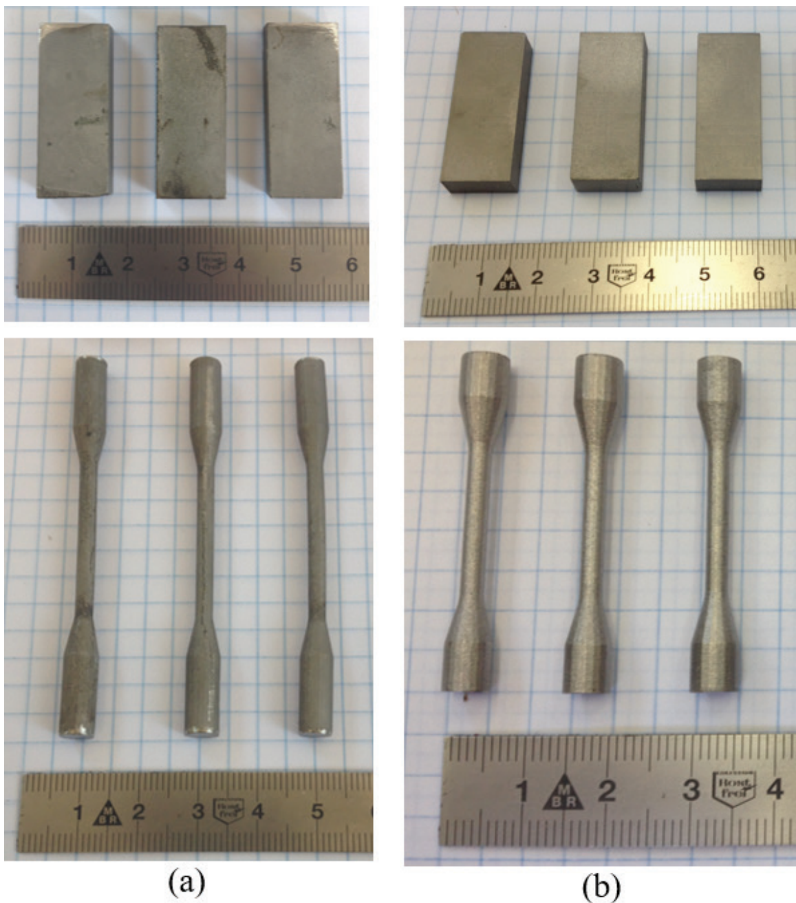
Figure 6. Specimens manufactured of Co-Cr-Mo alloy: (a) specimens made by FP technique and (b) specimens made by SLM technique.
