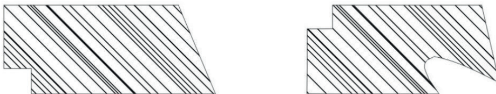
Figure 10. Second compression ring cross section.
