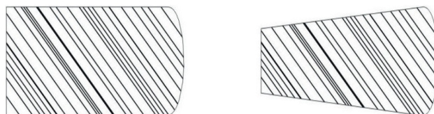
Figure 9. Top compression ring cross section.
