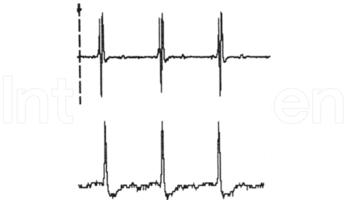
Figure 7. Raw and filtered electrograms sensed by a pacemaker. The top tracing is the filtered signal used by the pacemaker for sensing. Filtering of the raw signal is necessary to prevent (over)sensing of the T-wave, far-field signals, and myopotentials.
