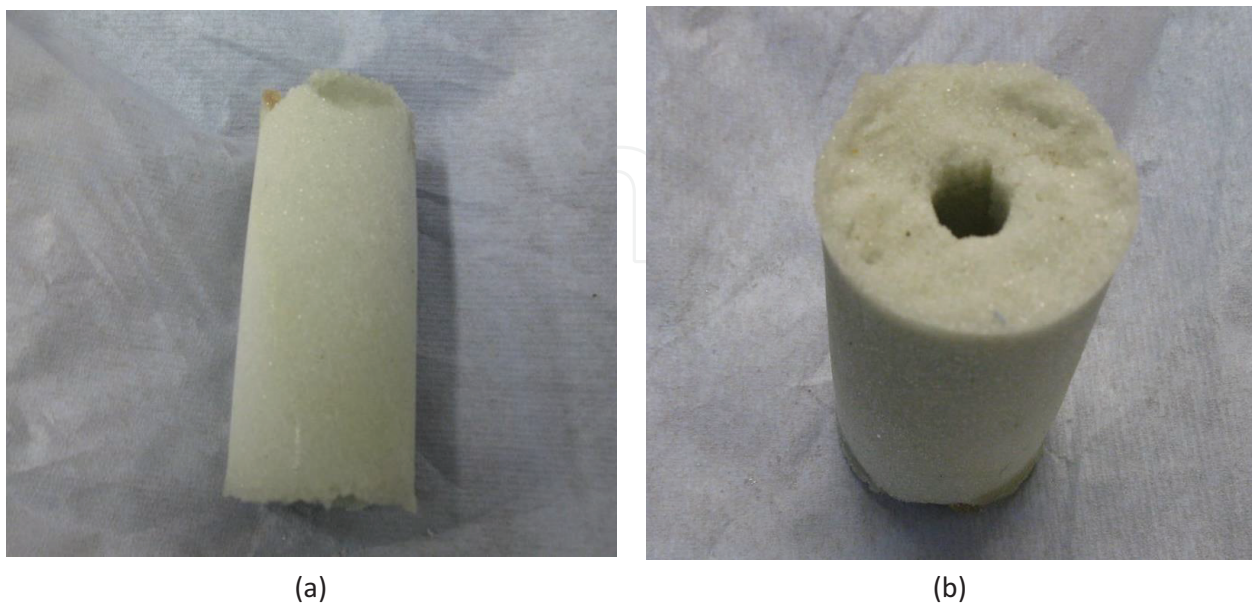
Figure 6. (a) A longitudinal view and (b) an oblique view of the synthetic rock (bonded glass beads).
