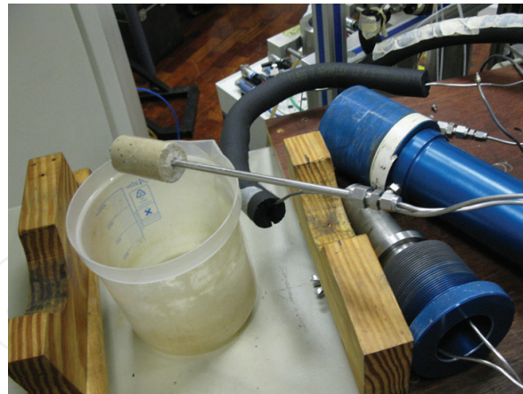
Figure 20. Experimental set-up showing the injection of fluid through a gypsum plaster specimen.
