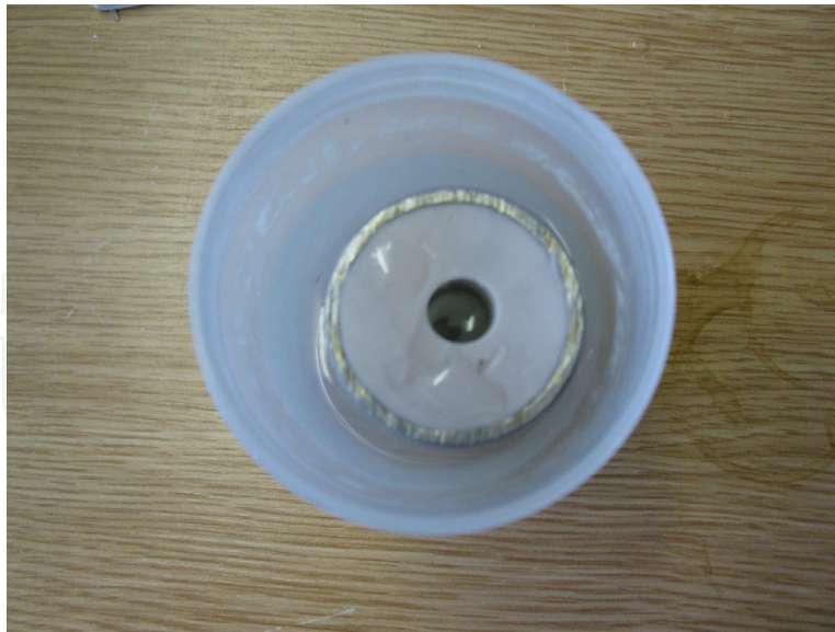
Figure 7. An immersed synthetic rock (luting cement), soaked in water before placement in the vacuum chamber.
