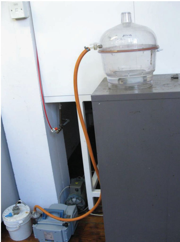
Figure 8. The saturation process and removal of trapped air using a vacuum chamber and pump.
