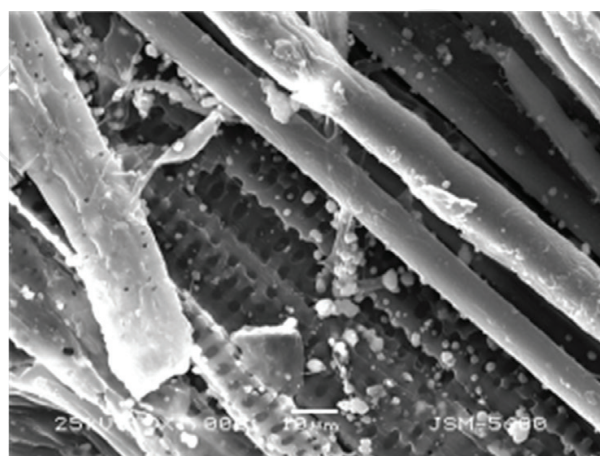
Figure 9. Morphologies of tensile fracture of (a) the bamboo fiber treated with alkaline solution; and (b) the untreated bamboo fiber.
