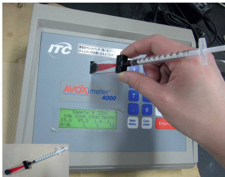
Figure 2. Portable oximeter (AVOX 4000) and its operation. Sample cartridge is shown in lower left-hand corner.
