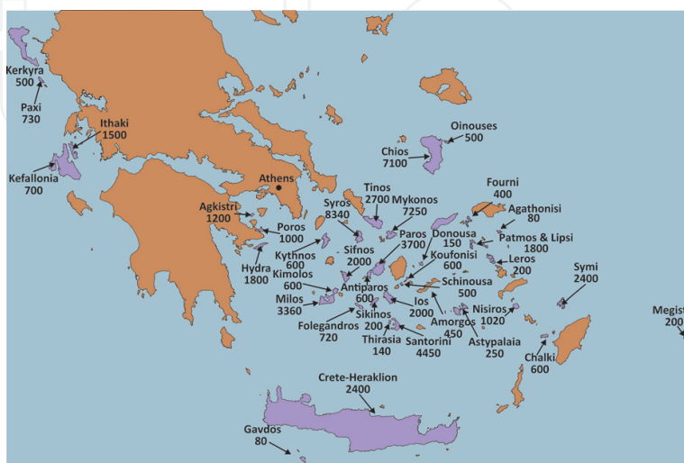
Figure 2. Desalination units in the Greek islands ([13, 16–22]; TEMAK SA, personal communication).
