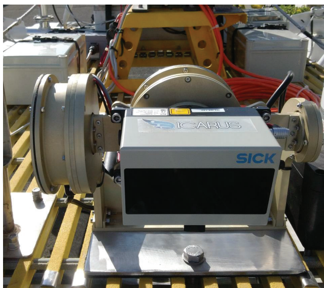
Figure 3. Laser scanner mounting platform and electronics (source: ICARUS).
