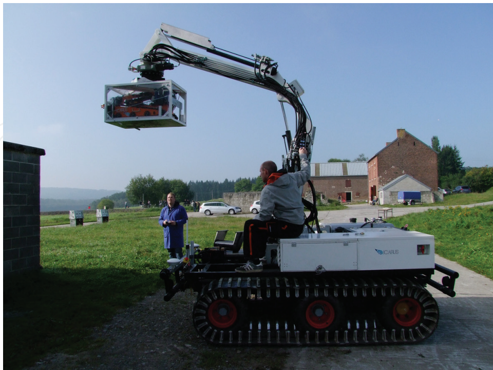
Figure 13. The LUGV uses its arm to lift the transport box containing the SUGV (Source: ICARUS).
