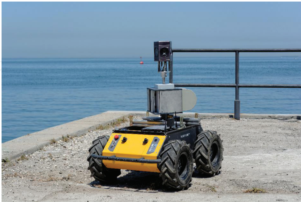
Figure 10. Dedicated support system—mobile mapping platform (source: ICARUS).
