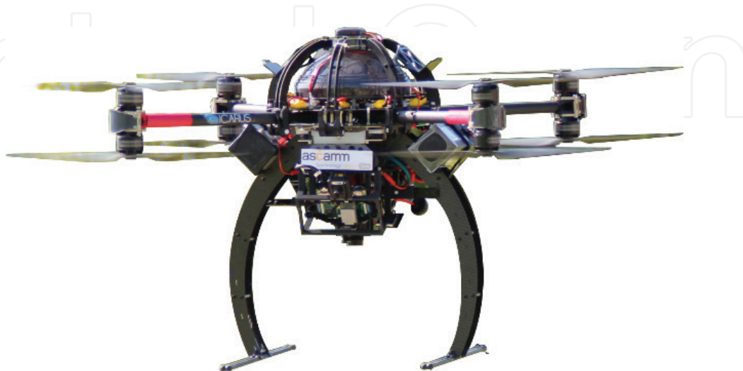
Figure 7. The Eurecat coaxial-quadrotor with the camera payload (source: ICARUS consortium).
