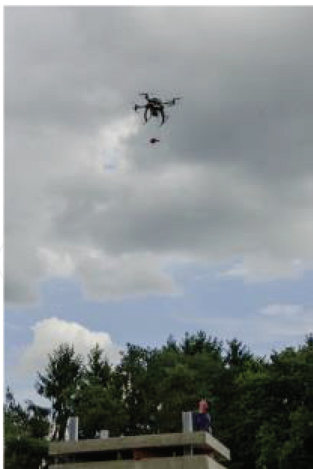
Figure 10. Eurecat quadrotor delivering a first aid kit to an injured victim (source: ICARUS consortium).
