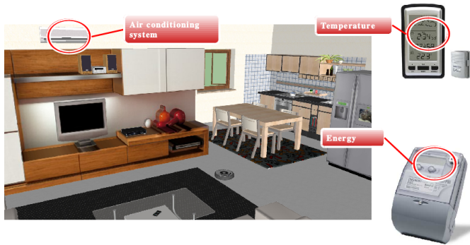
Fig. 3. Designed test scenario for this project. The scenario is composed of two sensors (temperature and energy sensor) and one actuator (air conditioning system).
