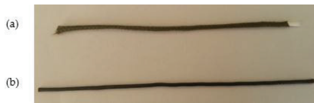
Figure 17. (a) Hybrid yarn before heating (b) Hybrid yarn after heating.
