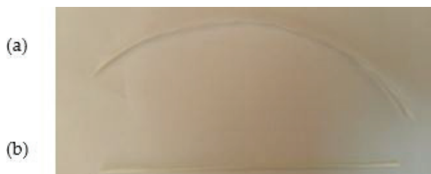
Figure 19. (a) Uncoated AR-Glass fibers (b) Coated AR-Glass fibers.
