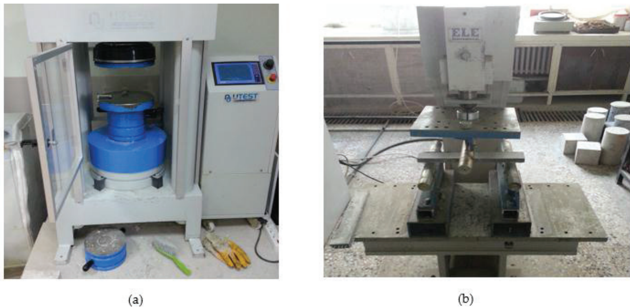
Figure 22. (a) Compression test machine (b) Flexural strength test machine.
