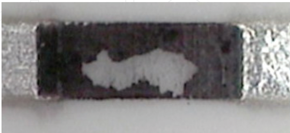
Figure 10. Photograph of catastrophically failed thick-film resistor due to the presence of hot spots caused by conducting material dispersion.
