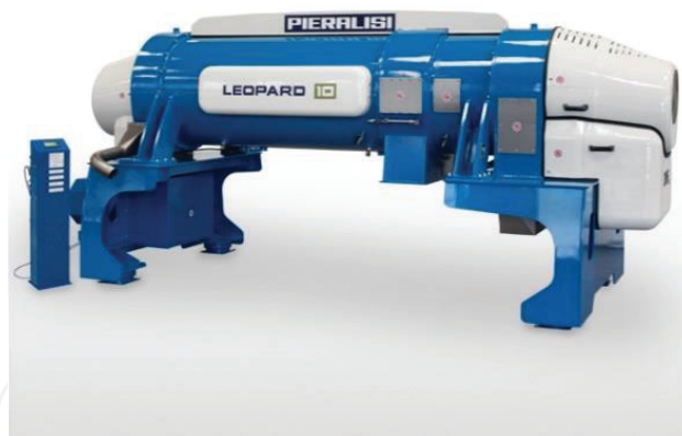
Figure 8. Last generation decanter extractors of olive oil, which combines the two-phase extraction technology without the addition of water with batch processing, thanks to the bowl discharging device. The installed power ranges from 7.5 Kw (more adapted to small quantities of olives to be extracted, i.e. process capacity of 0.5 tonnes/hour) to 45 Kw (for very large quantities of olives to be extracted, i.e. process capacity of 9 tonnes/hour) (Source: courtesy of Pieralisi SpA, Ancona, Italy).
