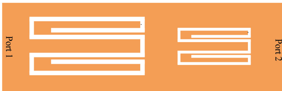
Figure 4. Configuration of the filter with two stop bands.
